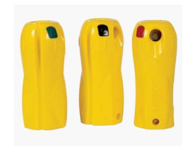
Marport's MFX Door Sensors use a master and slave configuration, communicating via a transverse wireless link on 110 or 144kHz. The master sensor interrogates the slave on the opposite trawl door, relaying data from both sensors to the catching vessel via a wireless uplink broadband transducer. As well as the
