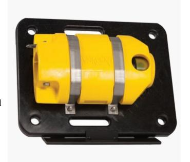
Marport's High-Definition Trawl Explorer is the skipper's eyes under the sea. Mounted on either the headline to provide a view of fish passing under it and back into the belly, or on the tunnel to show fish making their way down to the codend, the **HDTE** employs CHIRP technology to relay a detailed echogram image via a wireless link direct to the wheelhouse. It offers higher
