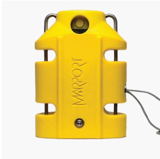
This downward-looking sensor is fitted on the top sheet of a codend or tunnel to allow the skipper to monitor the contents of the codend in real time as the gear is fishing, providing a series of updates on the fish as they pass into the codend from the trawl mouth and through the belly.
