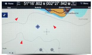
BUOY-Tracker is a fully certified AIS AtoN transceiver and correctly marks buoys as an AIS AtoN. This is in contrast to competing products which incorrectly mark buoys as vessels.
